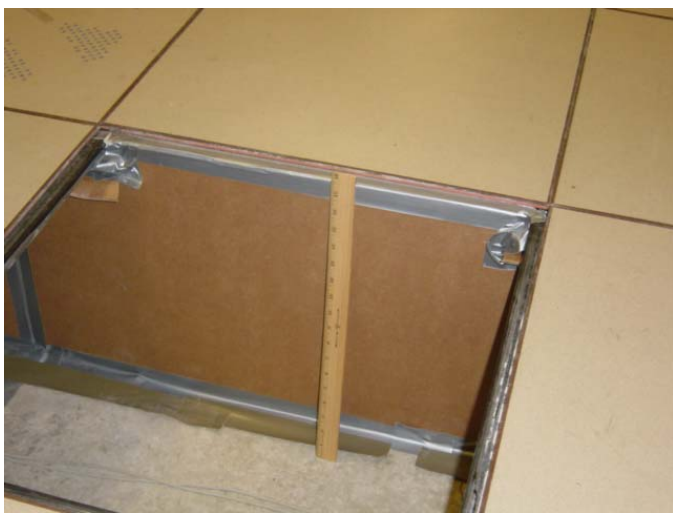
Figure 1. Cardboard partition used to seal the perimeter of the test area
